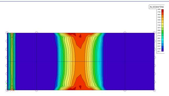
Figure : Required lower reinforcement - direction 2 (longitudinal direction)
