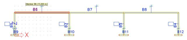
A PGNL calculation shows the adapted stifnesses Ely of the columns.
