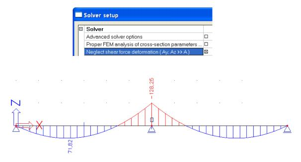
When we apply the non-linear calculation, the change of cross-section stiffness due to formed cracks results in a redistribution of internal forces.
