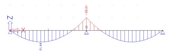
The bending moment calculated above the intermediate support is equal to 88.8 kNm.
