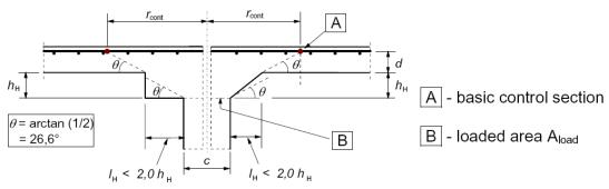
For a rectangular column with a rectangular head with  $l_{\rm H} < 2,0 h_{\rm H}$  and overall dimensions h and  $l_2$  ( $l_1 = c_1 + 2lH_1$ ,  $l_2 = c_2 + 2lH_2$ ,  $h \le l_2$ ), the value  $r_{\rm cont}$  may be taken as the lesser of:  $r_{\rm cont} = 2d + 0,56 \sqrt{l_1 l_2}$  and  $r_{\rm cont} = 2d + 0,69 h$
