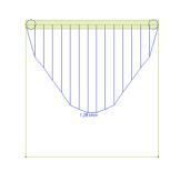
This can be explained by looking at the horizontal tension forces nx in the wall. In the picture below can be seen that the isotropic element will take the tension itself, so it is not transferred to the beam element.
