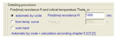
This can be adjusted in the setup for the entire structure but can also be overwritten for each beam by means of the Member Data (see later).
