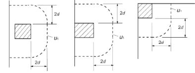
The value of d, the effective depth of the slab, is assumed constant and may normally be taken as:  $d_{eff} = (d_y + d_z)/2$  (EC formula 6.32)
