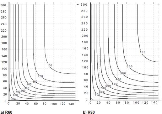
Figure A.7: Temperature profiles (°C) for a beam  $h \times b = 600 \times 300$
