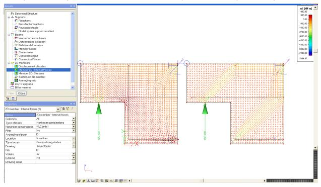
The pressure only walls show straight pressure lines that are only bended on the reinforcement ribs that will take the tension. To dimension these reinforcement ribs the normal forces working in these ribs can be asked. Based on these tension forces the user can dimension the reinforcement ribs. For the wall design the high tension forces that appear in the corner will be avoided. That is why this reinforcement configuration is a better design then a standard 2D reinforcement net.
