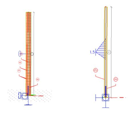
If we display the strain eps ct (concrete in tension) we see the following:
