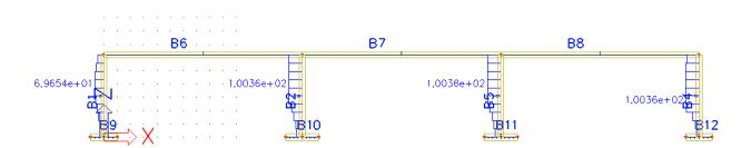
It is clear that reduced stifnesses are found on the bottom of the columns because there tension in the concrete is expected. This can be verified if we look at the tension strains in the concrete.
