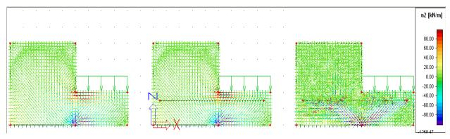
The reinforcement ribs are only effective if the concrete does not take any tension itself. To illustrate the normal force in the ribs is shown below.
