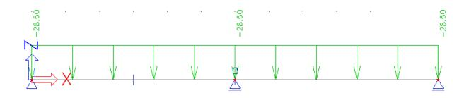
The linear calculation in SCIA Engineer gives the bending moment calculated above the intermediate support is equal to 127,6 kNm, which is very close to the direct solution.
