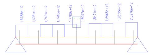
Pay attention to the number of mesh elements. If we had taken the default value of 1 element per beam, the stiffness was constant along the length. So, to obtain precise results the mesh has to be refined.
