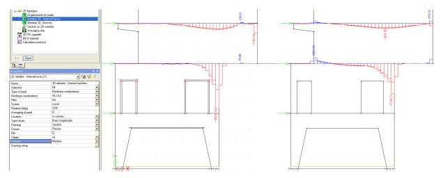
We can clearly see the effect of the pressure only wall in which the tensile forces are almost completely eliminated.
