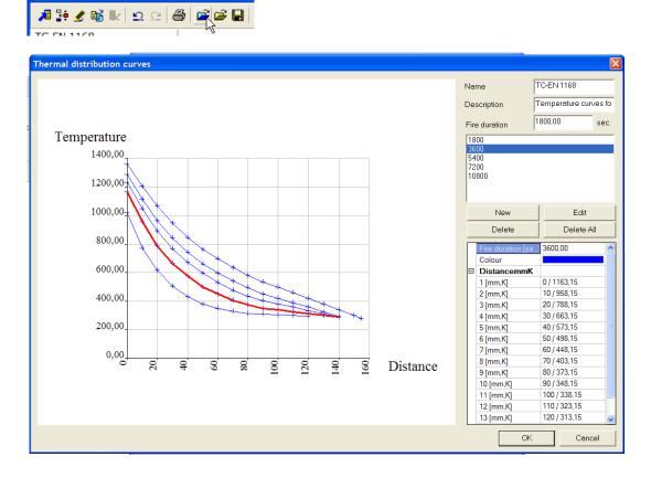
One temperature distribution curve defined in the temperature curves manager may in fact consist of several individual curves. Each individual curve is defined for one time duration of fire.
