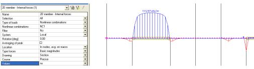
The tension in the horizontal direction also leads to tension reinforcement in this direction. It is visible that in the isotropic element the beam is not loaded but tension reinforcement is necessary.
